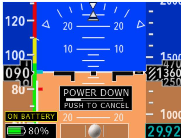
Figure 18 - On Battery Indication & Shutdown Timer
